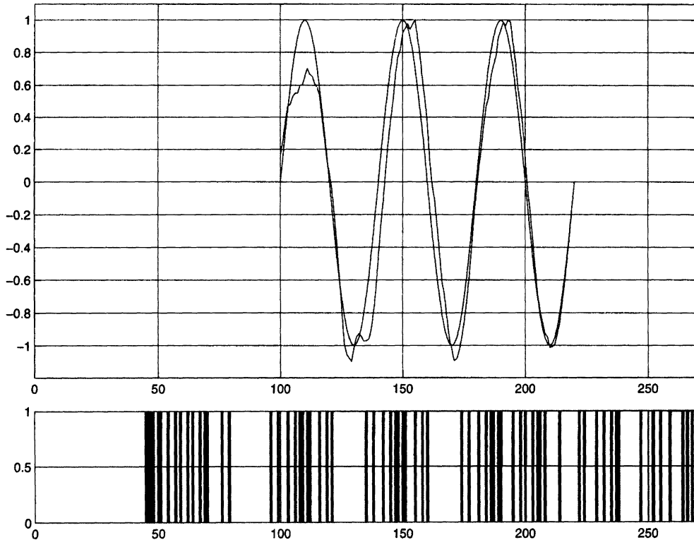
Figure 3. A 3 period sine curve resulting from convolution of an evolved CoDi-1Bit. The lower figure shows the actual spikes that generated the waveform.
